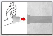
1. Simply insert the plug into the hole in the concrete wall with your hand.
