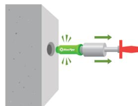
2. With help of the RiveOut, the RivePipe is removed from both sides of the wall
