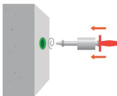
1. Once the wall has been stripped, the RiveOut is inserted into the RivePipe
