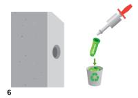
Expel the RivePipe from the RiveOut performing the counterweight action again, but now, in the opposite direction to the extraction. Keep the Rivepipe for your next reuse. The formwork tie hole remains now clean and homogeneous, and prepared to be sealed with RiveStop
